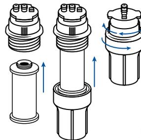
**5 Press new replacement filter** to the top of the filter housing using the appropriate color coded filters. Then, reconnect the bottom of the filter housing to the top half. Ensure connection points are correctly aligned, then turn clockwise to tighten. Continue this step for the second filter housing.
