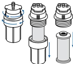
**NOTE:** If filter housing is too tight to disconnect by hand, please use the plastic wrench included with original system.
