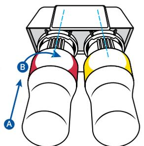
**7 Open battery door** and remove old battery. Insert new battery. When inserted correctly, system will beep five times and blink red.
