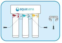
**2** Mark wall placement for mounting screws using built-in bracket on back of manifold. Make sure holes are as level as possible. Mark screw placement of the remineralizer holder 1 or 2 inches from the third stage sump to the right of the manifold.
