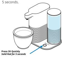
5. While red light is illuminated, press and hold dock button for 1 second. Light will blink red. While system flushes, light will continue to
