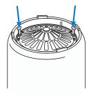
2. Remove the top tank snap ring. Remove the top cap from the housing assembly. Pull the cap out of the top of the tank by lifting up on the handles.
