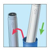
4. If necessary, clean the inside of the blue housing with mild soapy water, rinse and dry. Inspect o-ring for any damage and replace if needed.
