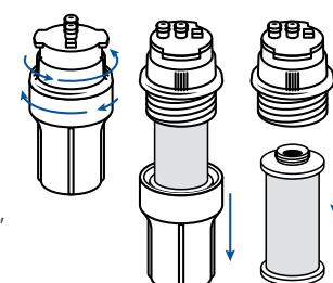
**3 Remove each filter housing** from the system manifold by turning the filter housing to the left. Pull down to detach. Ensure the filter housings are not on an angle while removing. This may result in damage to the o-ring.
