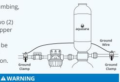
**ELECTRICAL SHOCK HAZARD** Prior to installation on metallic plumbing, securely install two grounding clamps and a #4 copper wire per installation instructions. Failure to follow these instructions can result in death or electric shock.
