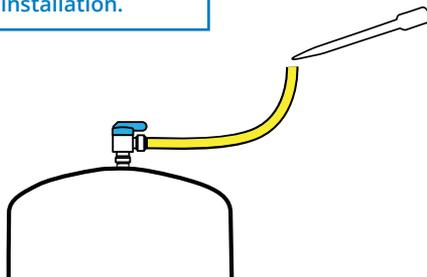
**NOTE:** Keep yellow tubing upright so that bleach does not spill or leak.
