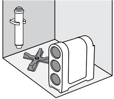
**NOTE:** Placement of bracket must be close to system manifold to ensure tube length needed for connection is sufficient.
