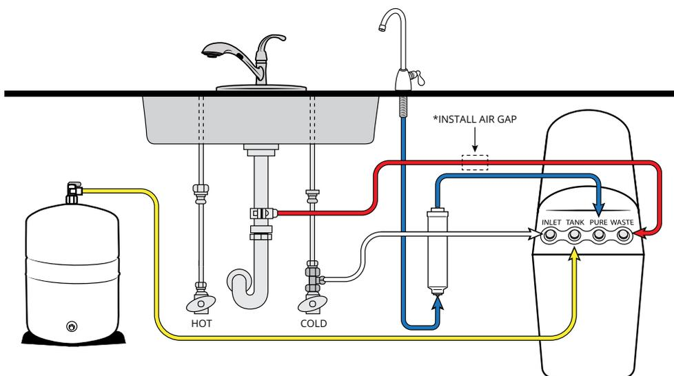
\*Properly install air gap to comply with local codes. Air gap must be two pipe diameters or 1 inch (25mm), whichever is larger.
