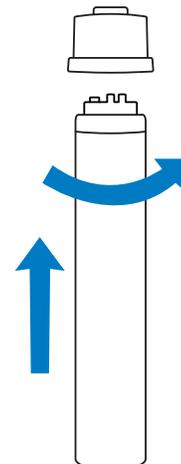
**NOTE:** Do not use tools to tighten. Hand tighten only.
