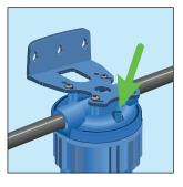
Remove the blue housing by turning the lower ring to the left, using the wrench supplied with your system. Remove the used filter and discard.
