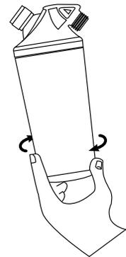
3. Unbox the replacement filter and remove the plastic. Then remove the yellow pull tab label and yellow plastic shipping cap from the top end of the filter.
