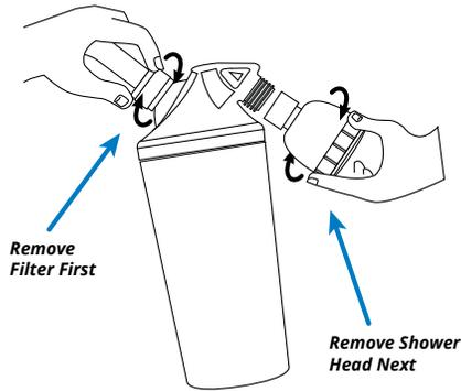
1. Remove the entire filter system from your shower pipe by turning the chrome swivel to the left. Then remove the shower head by turning the connector to the left.
