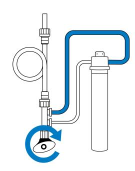
Remove the old filter from the system head. Rotate the filter to the left until it unlocks, pull down and discard.
