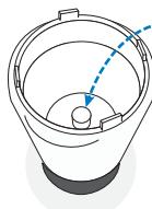
2. Press down on the cartridge so that the double O-ring seal moves into place within the bottom, center opening.
