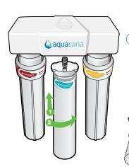
Attach new membrane filter to the bottom of the system manifold. Ensure connection points are correctly aligned, then push the membrane up while turning to the right. Ensure the membrane is locked in place, not on an angle, and is aligned as pictured.
