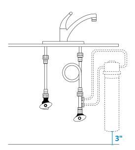
Three (3) inches of clearance from the base of the filter is needed for easy cartridge replacement.
