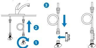
**NOTE:** Do not over tighten dual port adapter as this may result in a restriction of water flow.
