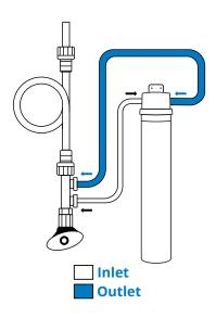
**NOTE:** Use 3/8" quick connect elbows in each port on the system head if necessary.
