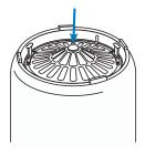
3. Release the red button and inspect the system for leaks. After inspecting for leaks, allow water to run through the system for 10 minutes for the final flushing period.
